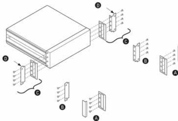
**Figure 2** Kits for Handles and Rackmount Flanges
