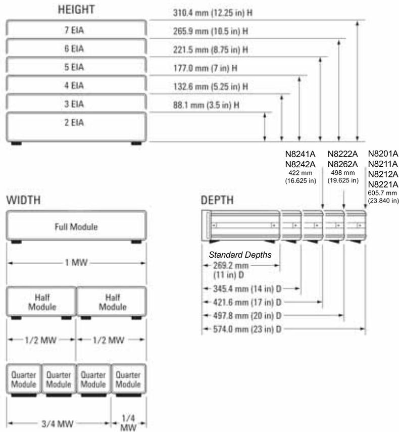
Figure 1 Height, Width (Module Width or MW), and Depth of System II Instruments
